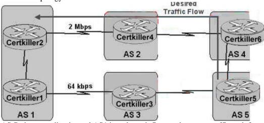
AS-Path prepending is used AS1 in order to influence the return traffic path from AS 5 to AS 1 through the higher speed via AS 2. \_\_\_\_\_\_\_ needs to be configured for AS-Path prepending and a minimum of \_\_\_\_\_\_ of the AS number should be prepended.
