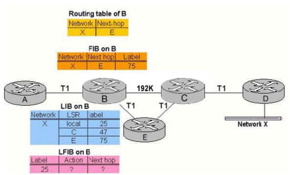
Refer to the graphic. At router B, complete the LFIB for a label of 25.
